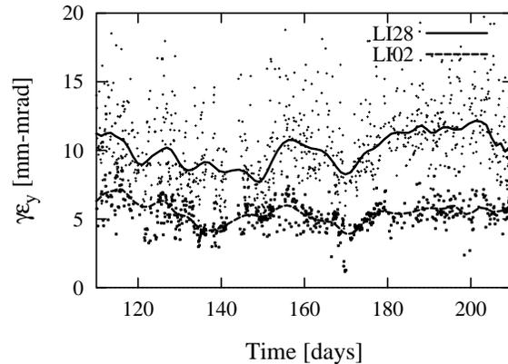
**Figure 7** Measured vertical emittances against time for the beginning (LI2) and end (LI28) of the SLAC linac. The data covers the period from April 1<sup>st</sup> to July 31<sup>st</sup>.
