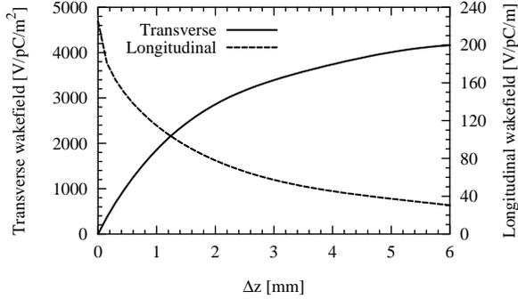
**Figure 2** Calculated transverse and longitudinal wake-field functions for the SLAC [1].
