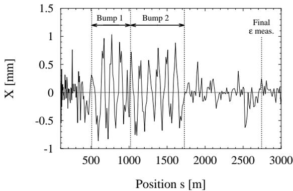
**Figure 5** Horizontal linac trajectory with bumps during record luminosity on June 21<sup>st</sup>.
