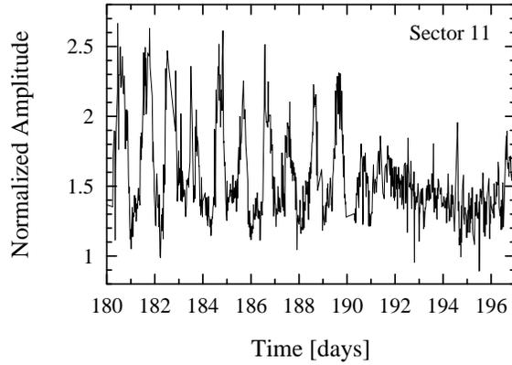
**Figure 9** Variation of the normalized amplitude of a betatron oscillation in sector 11 of the SLAC linac. A fix was applied on day 191 [5].
