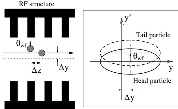
**Figure 1** Principle of a wakefield generated increase in the projected emittance. A single bunch is represented by two particles. The projected beam emittance is increased due to a wakefield kick  $\theta_{\text{wf}}$ .
