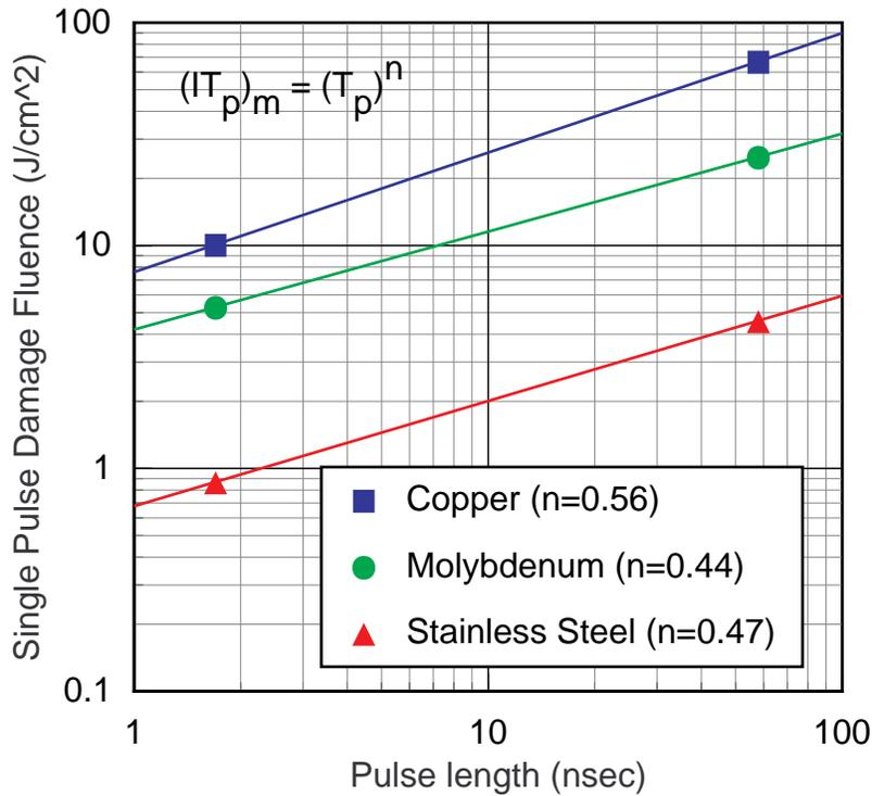
This was based on 100 pulses and extrapolation to a larger number is not meaningful. They measured this same dependence for mirrors prepared by different manufacturers using different surface preparation techniques and concluded that the failure was determined by intrinsic properties of copper.
