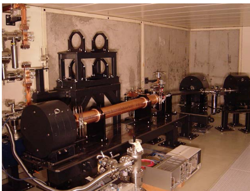
Figure 16. High-power setup for C-band accelerator structure testing at SPring8.
