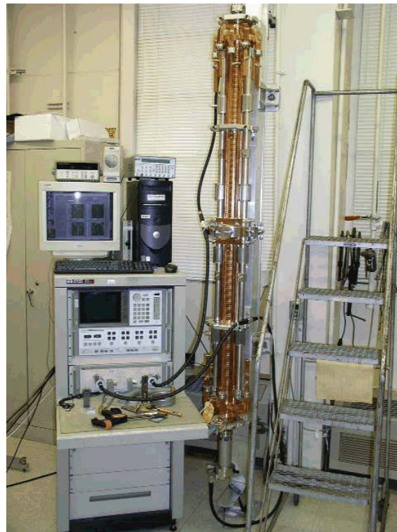
Figure 12. Wire measurement set-up with the RDDS1 Structure.
