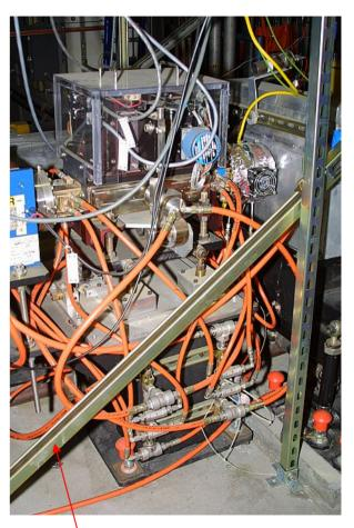
Unistrut bracing to shield wall may need to be temporarily removed to enable hoist access to collimator
