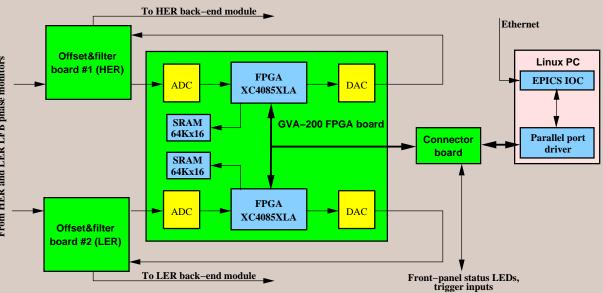
The LGDW prototype implements a 14 tap FIR filter, with a 9.81 MS/s processing rate.
