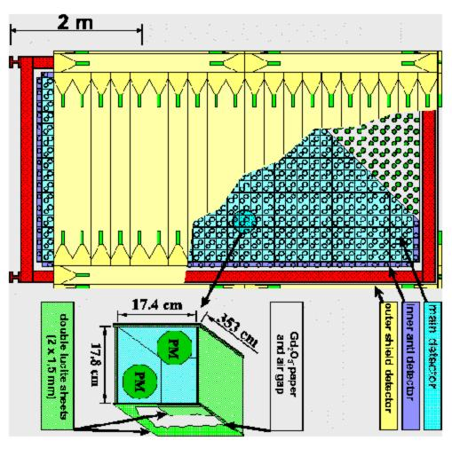
512 modules of liquid scintillator with Gd<sub>2</sub>O<sub>3</sub> for neutron capture
