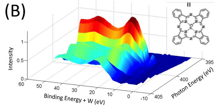
**Resonant Electron Spectroscopy** shows that donor/acceptor electron transfer is faster at face-on vs. edge-on orientations. (A) Cartoon illustrating the relative orientations between the Cu phthalocyanine donor (blue) and  $C_{60}$  acceptor (black). (B) Resonant Auger electron spectra, which were used to measure the branching ratio of Auger electron decay processes. This branching ratio is related to the average time it takes an electron to hop from the excited donor to a nearby acceptor.
