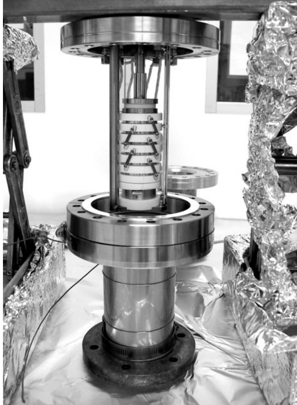
A Purity Monitor for Liquid Xenon Used in EXO.
