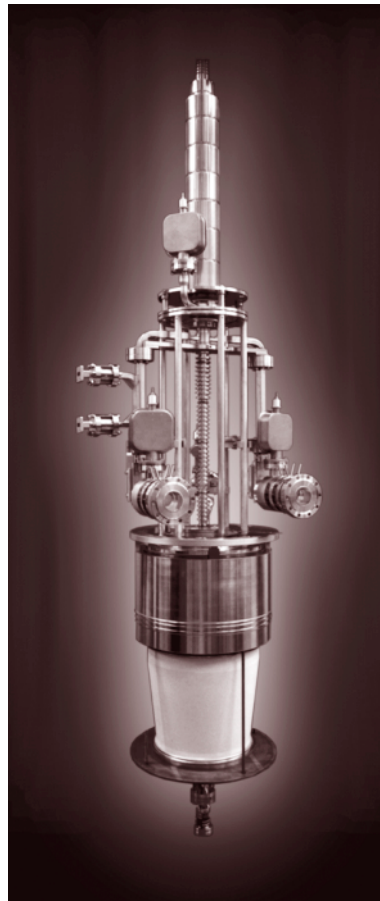
A 75 MW Prototype Klystron Producing 11.4 GHz rf Power for the Linear Collider R&D Program.
