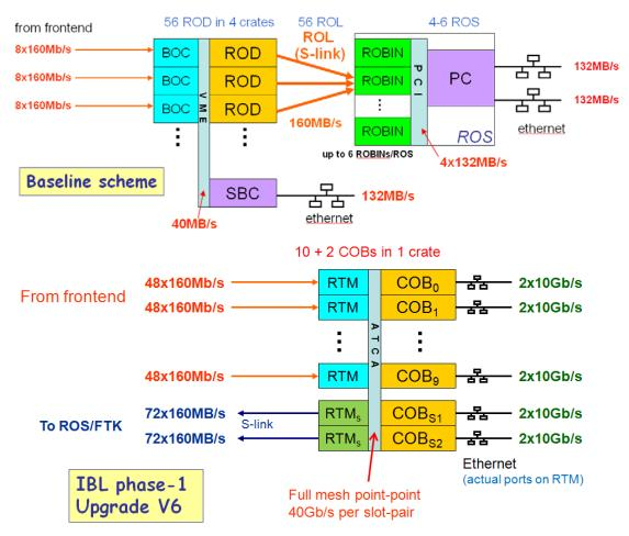
Figure 5: Comparison of the system configuration using the existing RODs (top) and new RCEbased COBs located in an ATCA shelf (bottom).
