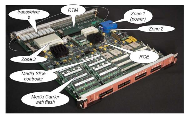
Figure 1 The RCE board. (The Media Slice controller and Terabyte of flash memory are only relevant to the PetaCache project.)
