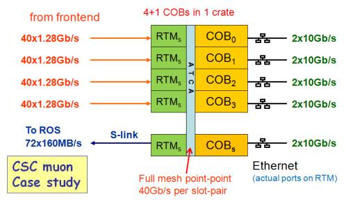
Figure 8: CSC muon readout replacement with RCE-based COBs.
