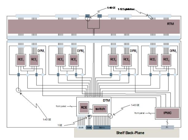
Figure 3: Block diagram of the Cluster-On-Board (COB). Each Data Processing Module (DPM) contains two RCEs. The Data Transportation Module (DTM) contains a single RCE, capable of functioning as a TTC emulator. The IPM Controller (IPMC) manages and monitors the board's configuration.
