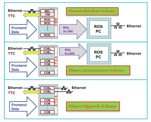
Figure 9: A possible evolution path for a pixel readout crate and corresponding ROS processing. In all scenarios, each COB has its own 2x10GE *Ethernet* ports which are not all drawn.
