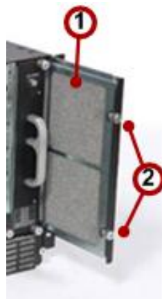
Figure 26: Air Filter Removal for Inspection
