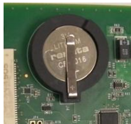
Figure 26: Shelf Manager Board Battery
