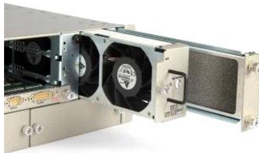
Figure 24: Air Filter Removal for Inspection
