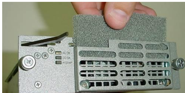
Figure 25: Replacing the Power Supply Filter
