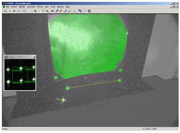
The crosses represent points that have been located in this particular image. Note that the image appears a little dark and difficult to see. This is intentional as the best photogrammetric measurements are made on images that have dark backgrounds and bright targets. Some of these targets are shown in the zoom window in the corner. If the scale bar is visible then a yellow line will be drawn between the two end points.
