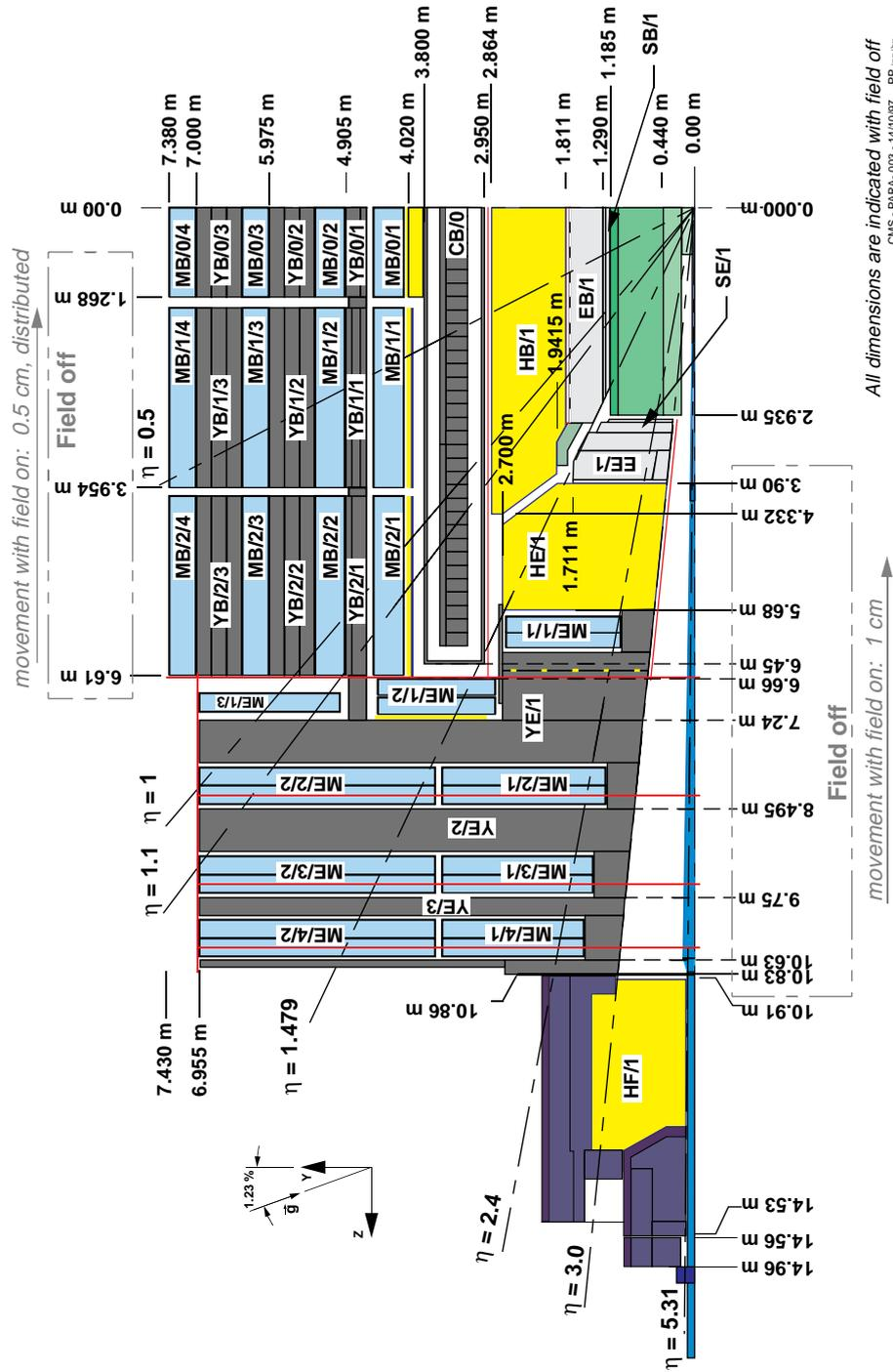
Figure 1 –CMS longitudinal view: On green the central tracker, on white and yellow the calorimeters and on blue the muon spectrometer
