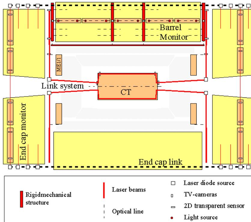
Figure 3 Longitudinal view of a active plane. The MS and CT volumes are shown with the alignment reference lines created by the different alignment subsystems.
