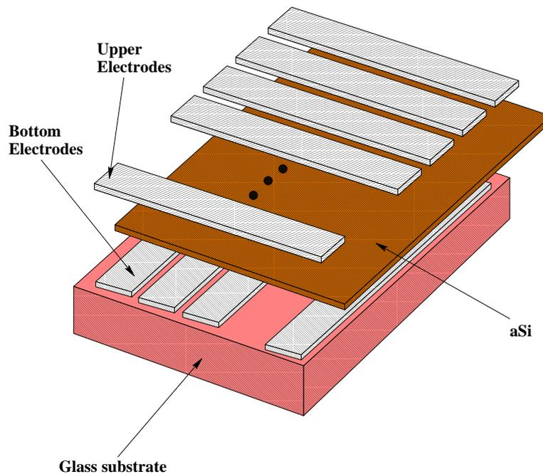
Figure 1 – 3D pictorial view of an ALMY sensor.
