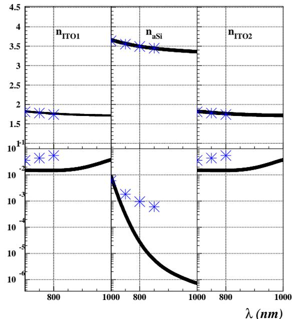
Figure 10 – Real and imaginary components of the refractive index of ITO (upper electrodes), a-Si:H and ITO (bottom electrodes). Asterisk are the mono-layer starting values for the simulation. The line represents the calculated value. The set of  $(n,k)$  shown here reproduce  $T$  and  $R$  as shown in Figure 8 and Figure 9.
