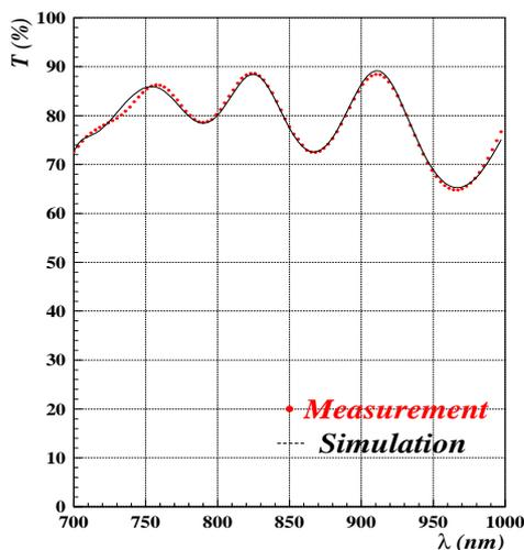
Figure 8 – Transmittance for the system ITO + a-Si:H + ITO + glass substrate. The effect of a finite size substrate is also included as in Figure 8.
