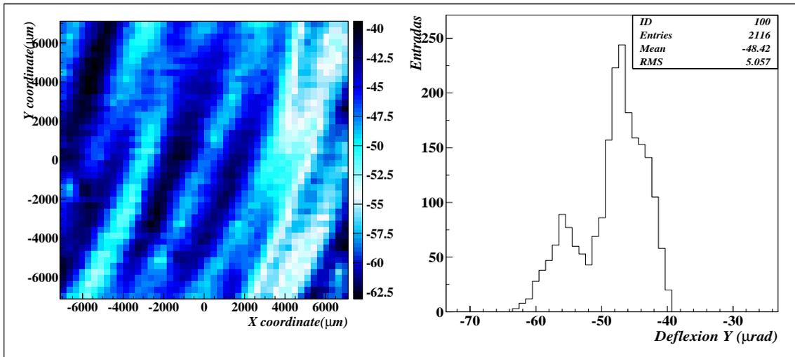
Figure 6 – Scan ( $312 \times 312 \mu\text{m}^2$ ) of one ALMY sensor type II, as seen by a CCD camera. The sensor shown is not that in Figure 3.
