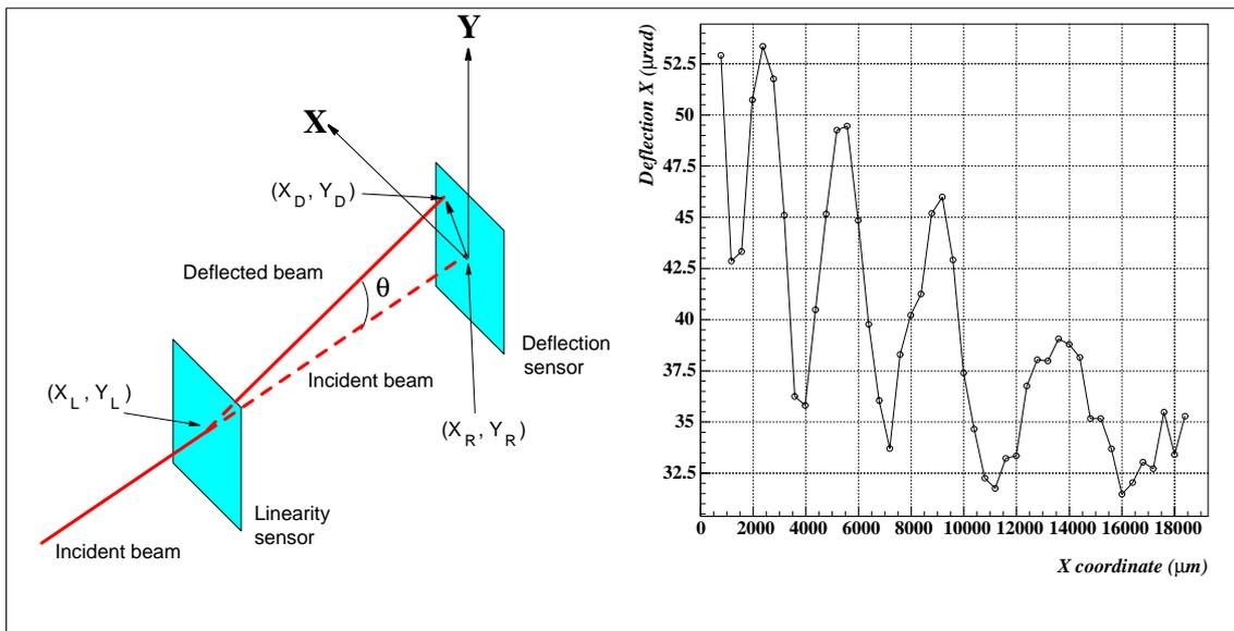
Figure 4 – Deflection measurement procedure.
