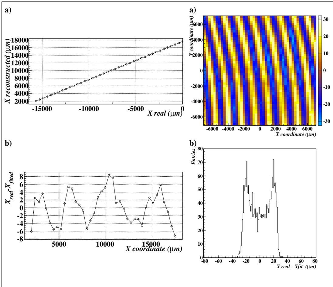
Figure 2 – a) Reconstructed position along a 1D scan of a sensor. b) Residuals of the linear fit.
