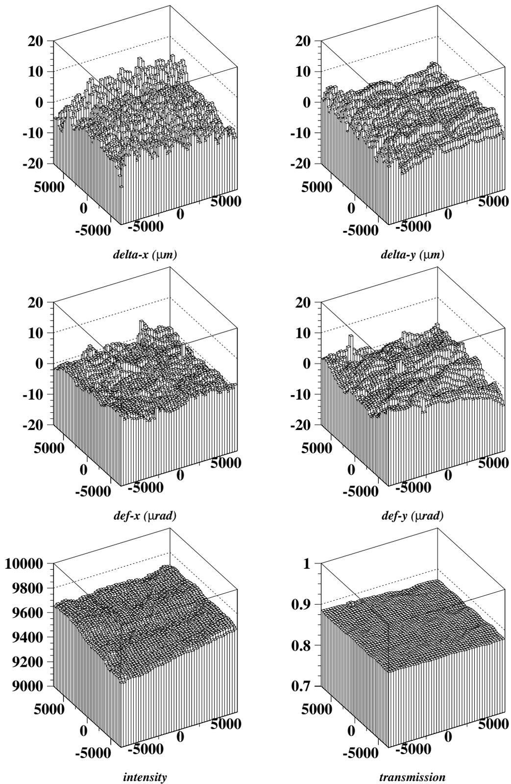
Figure 11 – Performance of the new ALMY type II sensor. From top to bottom, left to right: spatial uniformity X, spatial uniformity Y, X and Y deflection distributions, integrated photocurrent and transmittance.
