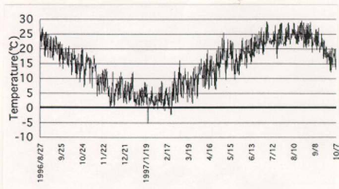
Fig.10. Temperature at the side wall of underpath.
