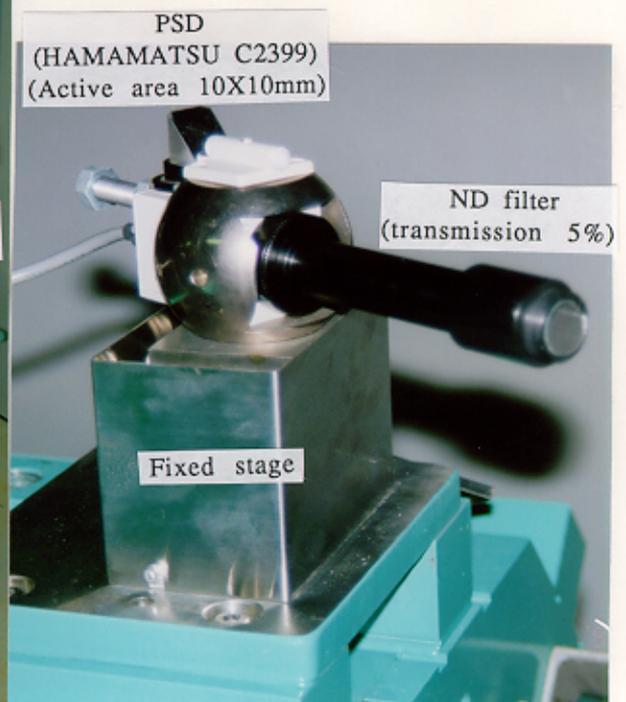
Fig.6. PSD Target.
