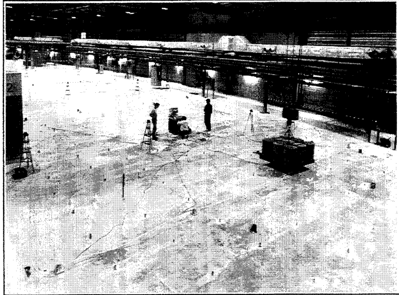
Fig. 14 Photograph showing the general setup used in the industrial measurement campaign of the ESRF EXPH slabs.
