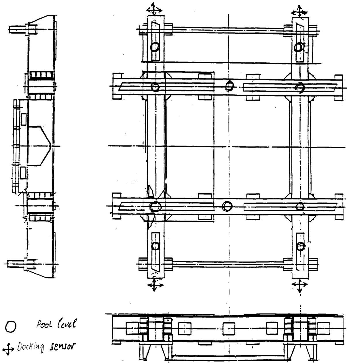
Fig. 2 The platform, with liquid level and docking sensor locations
