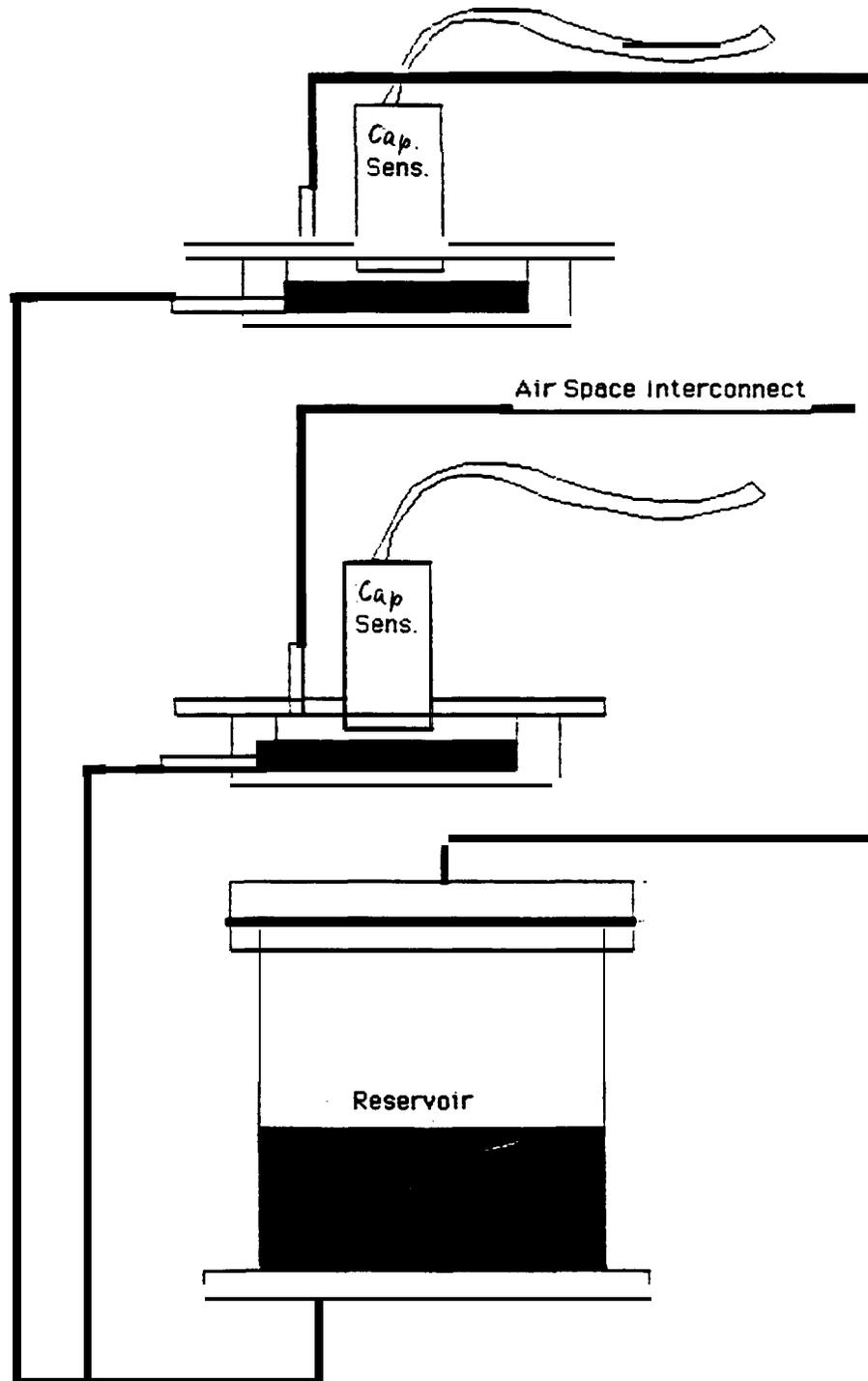
**Fig. 5 Schematic of as Liquid Level System**
