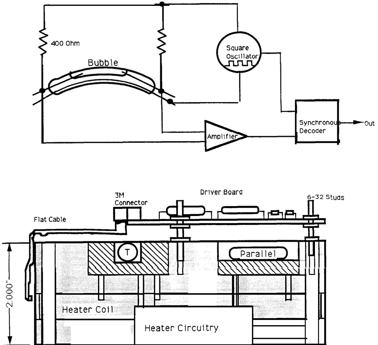
**Fig. 9 Tiltmeter Block and Schematic**
