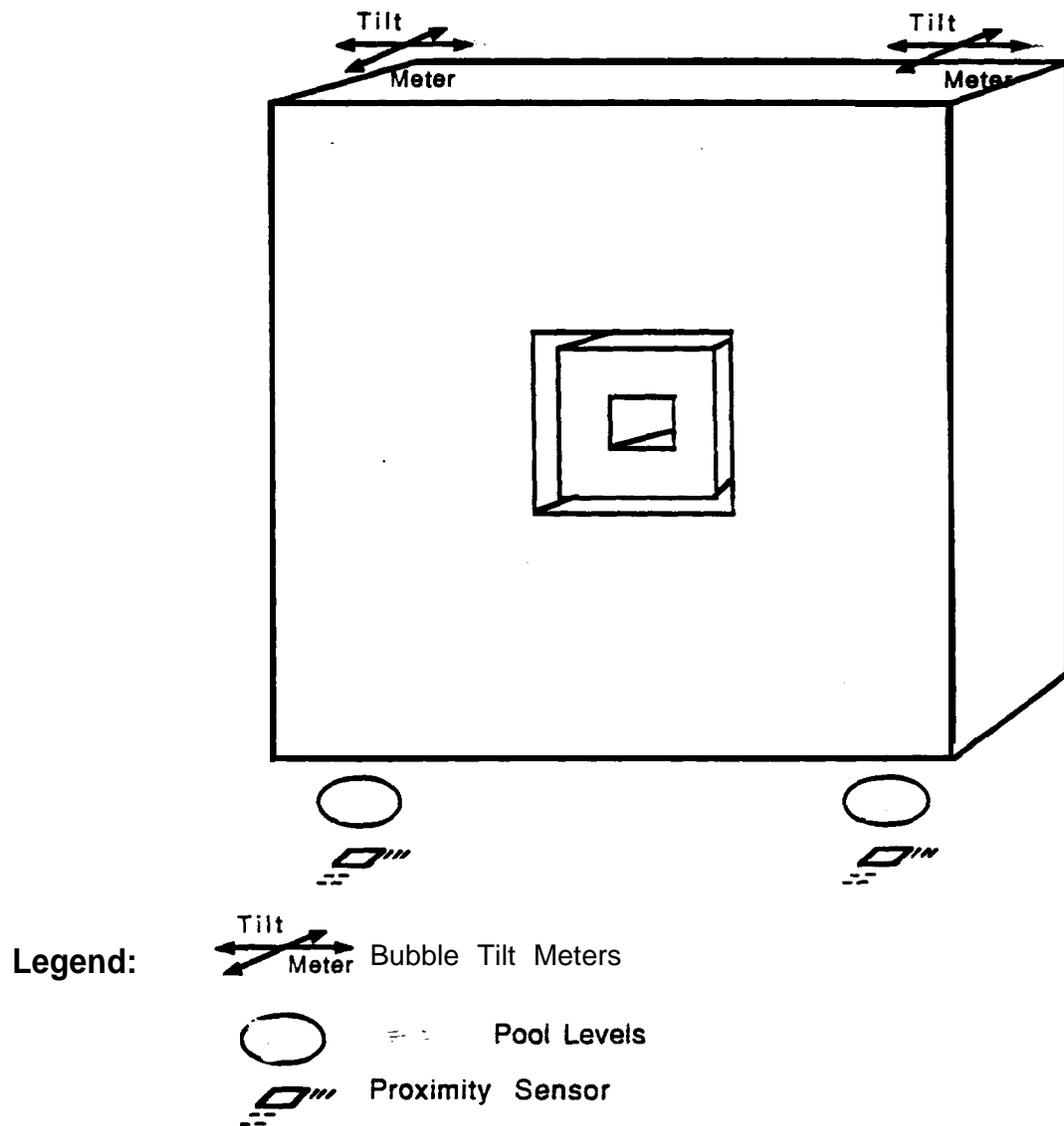
**Fig. 4 Tiltmeters and Liquid Level Sensors on the End Iron**
