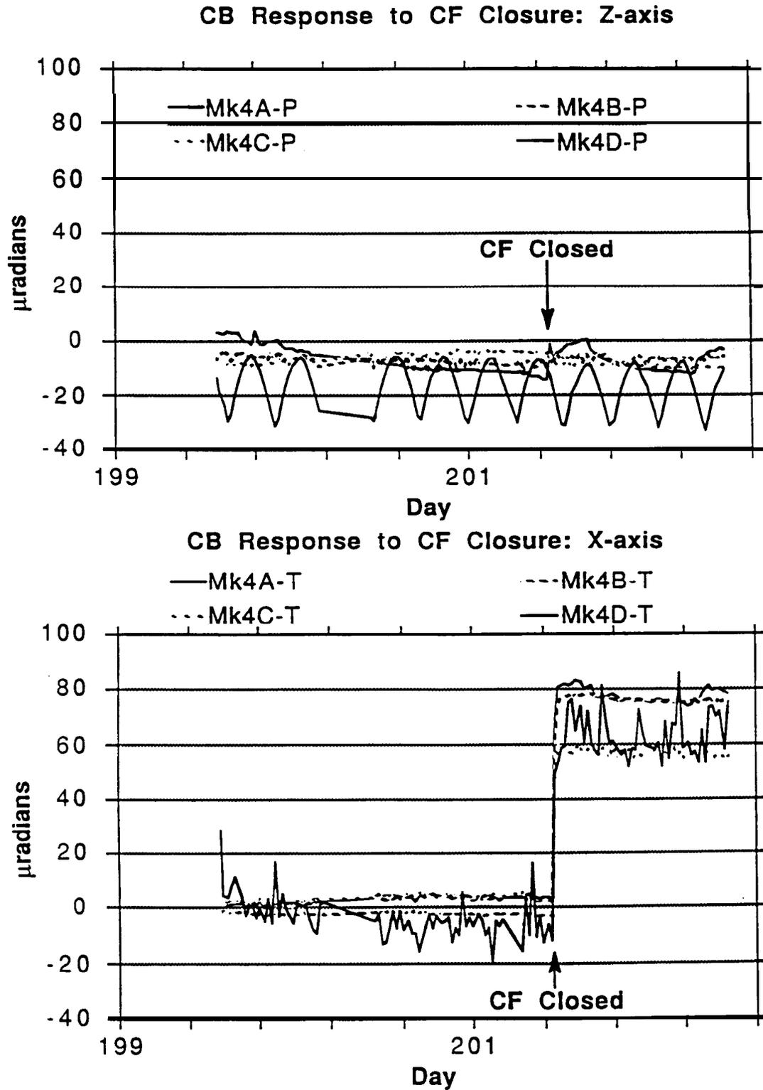
**Fig. 11 Response of the P and T Sensors on the Central Beam during Central Iron Closure**
