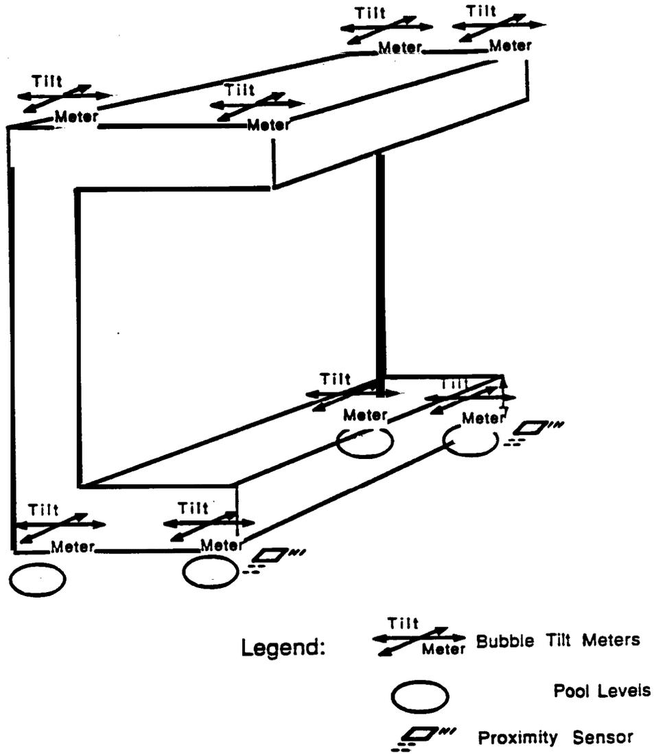
Fig. 3 Tiltmeters and Liquid Level Sensors on the
