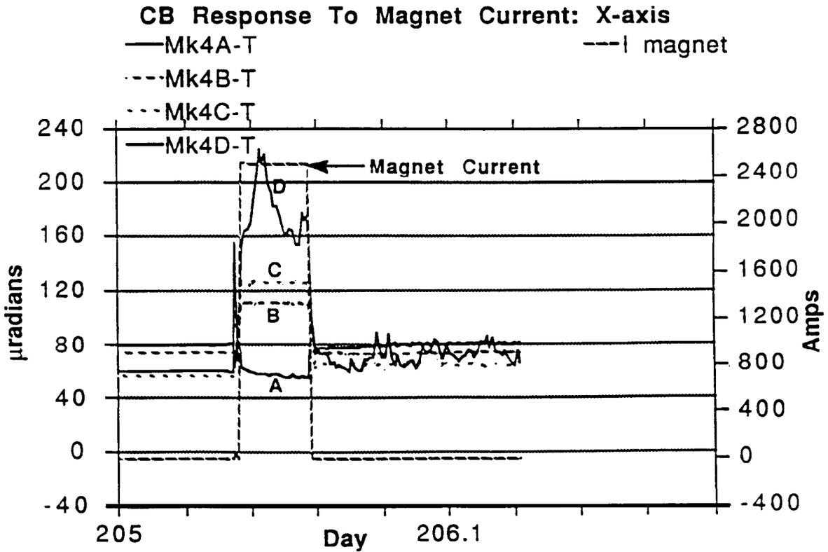
Fig. 12 Response of the P and T Sensors on the Central Beam during Magnet Excitation
