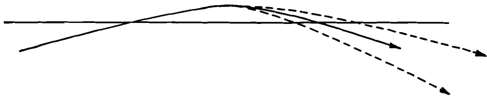
Fig. 6. Illustration showing effect of multiple scattering on muon trajectory.
