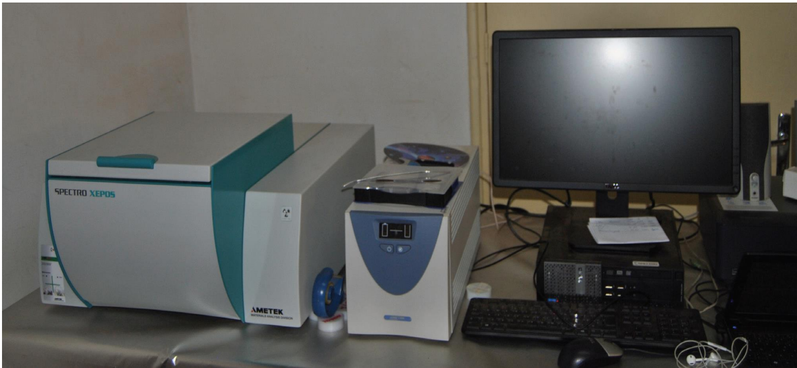
Figure 5. X-Ray Fluorescence analysis at INSTN-Madagascar laboratory
