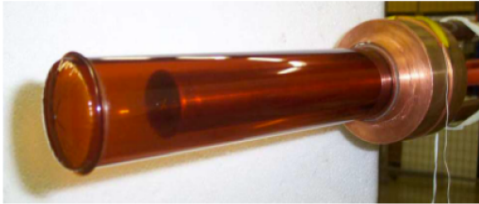
Kapton cell for liquid hydrogen target
