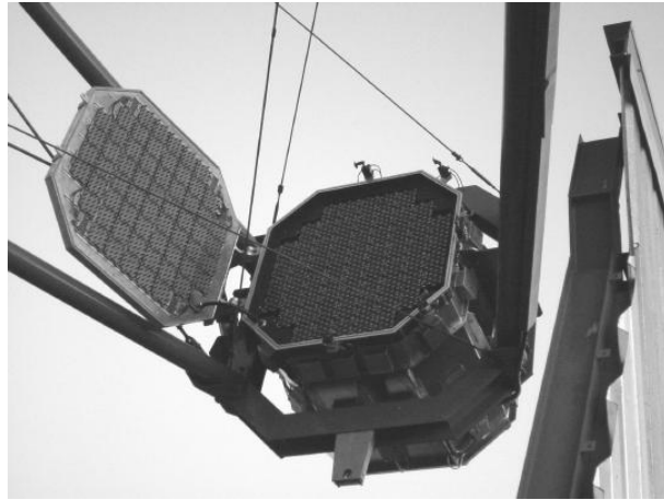
Fig. 3. Camera and related front-end electronics mounted at the focal plane of the telescope. Only three interconnect cables are needed to communicate with the DAQ System of H.E.S.S.
