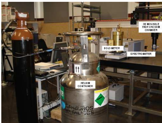
Figure 1: The spectrometer, the 3D movable high vacuum chamber, the silicon bolometer and the helium container
