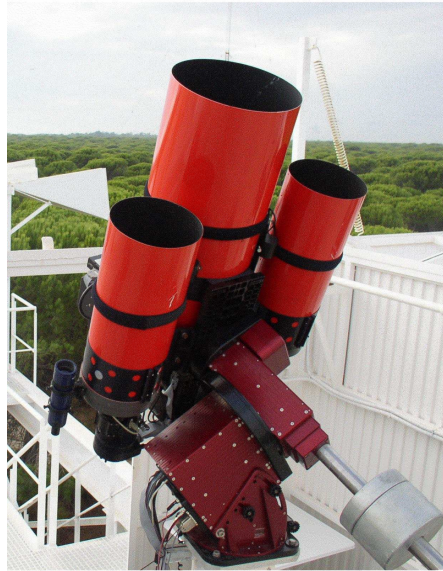
Figure 6: The BOOTES-1 0.2m and 0.3m diameter telescopes at Instituto Nacional de Técnica Aeroespacial in Mazagón (Huelva). They will be replaced by a 0.6m telescope.
