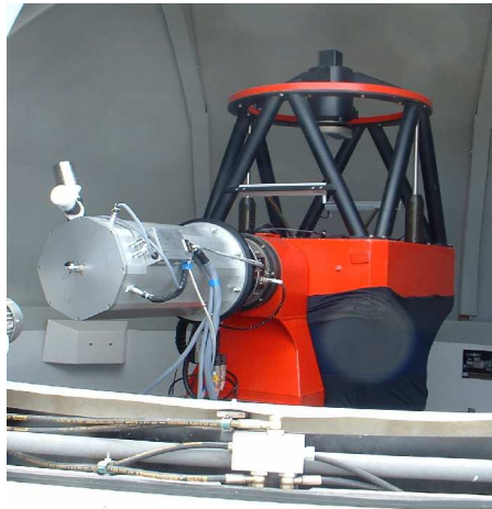
Figure 8: The BOOTES-IR camera (BIRCAM) attached to the 0.6m robotic BOOTES-IR telescope at the Observatorio de Sierra Nevada.
