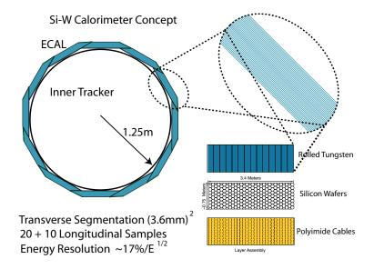
Figure 1: Silicon-tungsten ECal as envisioned for the SiD concept.
