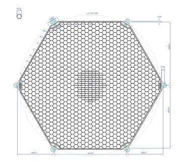
Figure 2: Schematic of version 2 silicon sensors. The central region includes a pad array to which the KPiX ASIC is to be bump or gold-stud bonded.
