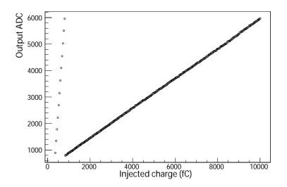
Figure 3: KPiX output as a function of input charge, showing the dynamic gain change at about 700 fC.
