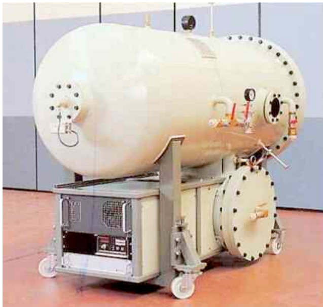
CW proton accelerator for {}^7\text{Li}(p,\gamma){}^8\text{Be} monochromatic \gamma 17.6MeV
