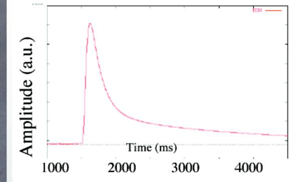
$T_0 \sim 10 \text{ mK}$  Numerology: C ~ 2 nJ/K ~ 1 MeV/0.1 mK G ~ 4 pW/mK Need to be able to detect temperature jumps of a fraction of µK (per mil resolution on MeV signals)
