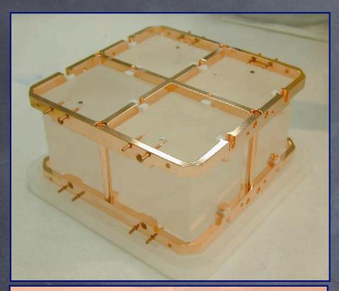
The bulk of Cuoricino calorimeter is made by 44 TeO<sub>2</sub> crystals of 5x5x5 cm<sup>3</sup> (790 gr of weight). There are 18 additional crystals of 3x3x6 cm<sup>3</sup> (330 gr)
