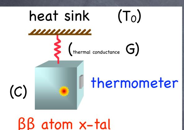
Basic Physics:  $\Delta T = E/C$ (Energy release/ Thermal capacity) Implication: Low  $C \Rightarrow$  Low T Bonus: (almost) No limit to  $\Delta E$  ( $k_BT^2C$ ) Not for all :  $T = C/G \sim 1s$
