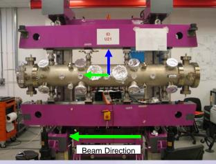
Final Assembly of Undulator 21, awaiting installation and final positioning inside the storage ring on ID Straight I03.
