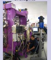
Faro Laser Tracker booked into Storage Ring controlled Network for final positioning of ID21. Careful adjustments are made to finally locate survey monument positions within 50µm against nominal data.
