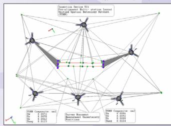
Typical instrument geometry and network configuration for the pre-alignment of both in and out of vacuum Insertion Devices. Uncertainty values of 12 to 15 microns (2.0 sigma) achieved for the positions of the survey monuments within the controlled
