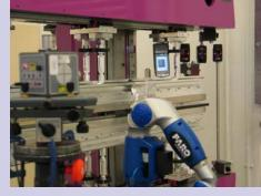
The ID's lower beam is set level to gravity with the Hamar system. Capturing the live data, columns are adjusted to bring the upper magnet array parallel and level to within 20 µm of the lower beam working surface (datum plane). Due to small working areas, the Faro Gage Arm is then introduced
