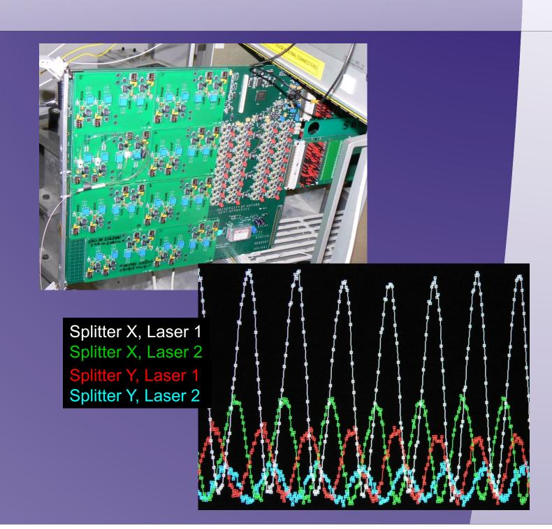
A multi-channel read-out system has been developed that uses sensitive avalanche photo-diodes (APDs) to detect the pW return signals. A series of 9U VME cards shown above each read out 64 fibre-coupled interferometers. The read-out is multiplexed so that signals from two optical switched interferometers reach one APD in alternate time slots. The plot shows four intensity signals for the two lasers and two GLIs that were read out successfully by one APD as the optical frequency was scanned.
