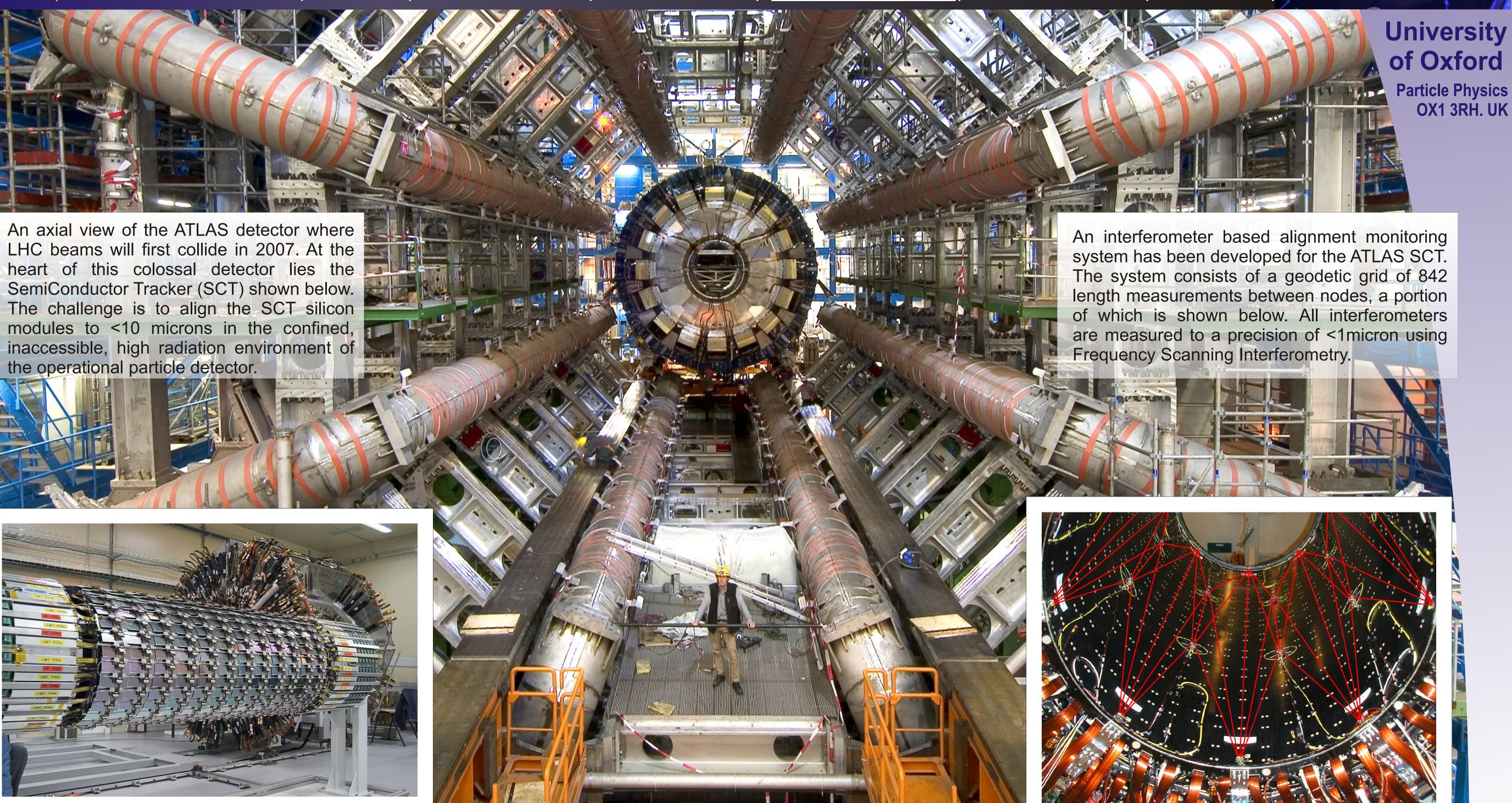
Frequency Scanning Interferometry is a technique for multiple, simultaneous and precise distance measurements in a hostile environment. A tunable laser illuminates a reference interferometer and multiple interferometers to be measured. As the optical frequency is scanned, a phase shift is induced in all interferometers, at a rate that is proportional to the length of each interferometer. The phase shifts are compared to determine the ratio of interferometer lengths to <1ppm.
