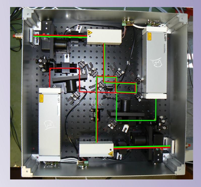
The above two-colour laser-amplier system illuminates all 842 interferometers. The two lasers are tuned in opposite directions to reduce the effects of drift in the interferometer length during a frequency scan, as shown in the plot below. The remaining error in the phase measurement is minimised by rapid scans and by scanning over a large frequency range. A precision of <100nm has already been achieved with this system.
