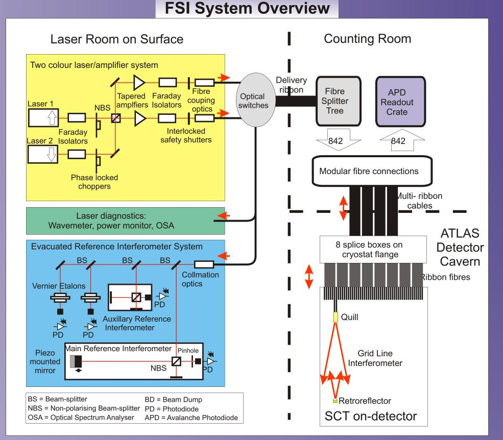
The laser light is conveyed to the GLIs via a fibre-splitter-tree of fused taped couplers. Recently available IR MEMs optical fibre switches enable the optical power delivered to the GLIs to be cost-effectively doubled. Tests in Oxford show precise FSI measurements using an active optical switch are possible, as plotted below.
