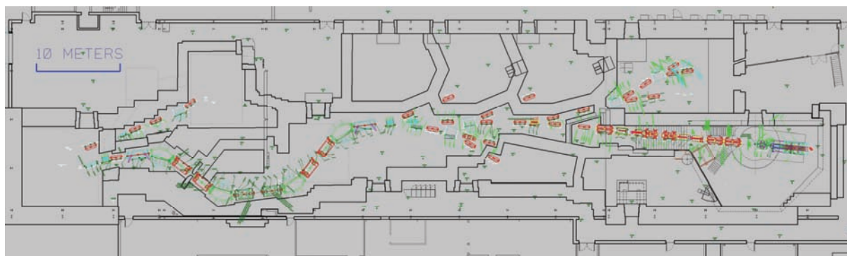
Figure 8. As-built laboratory layout from laser tracker measurements.
