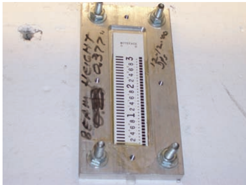
Figure 3. An optical tooling scale used as a vertical reference.
