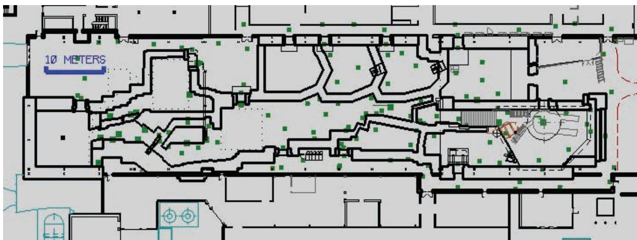
Figure 5. Locations of the laser tracker floor and wall monument grid points.
