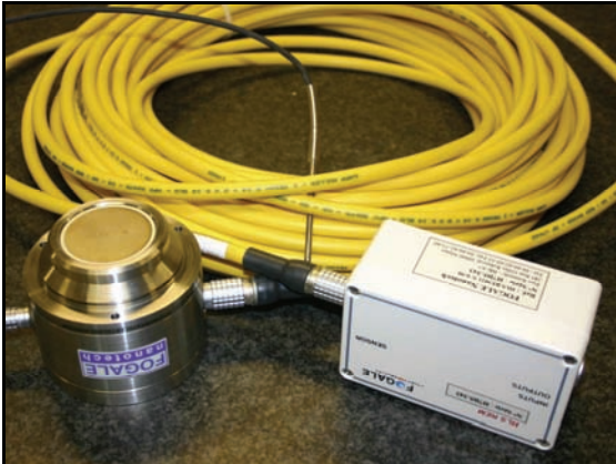
Figure 2: HLS sensor 4 th generation with remote electronic, temperature sensor and cable
