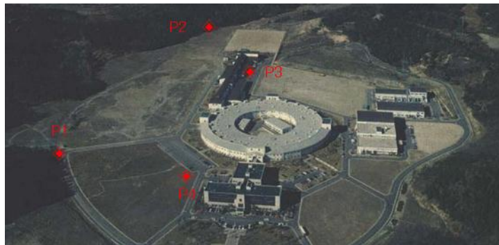
Figure 10: Survey posts for the absolute elevation measurement
