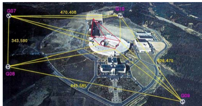
Figure 12: Distance survey for the outside survey network
