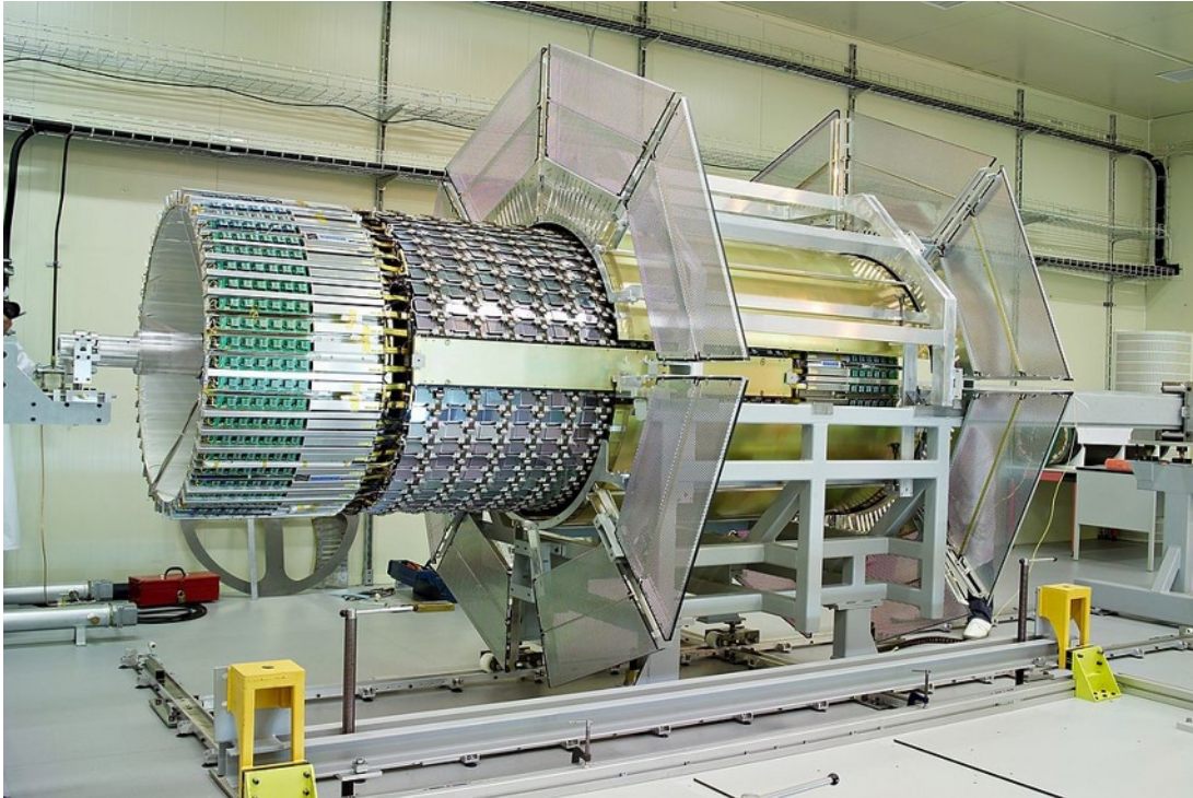
Figure 2: The S emi C onductor T racker lies at the heart of the ATLAS detector shown in Figure 1. The SCT Barrel is a \varnothing 1 m by 1.5 m long particle detector, pictured here during insertion of the largest cylindrical layer of silicon-strip detector modules into the outer thermal enclosure.
