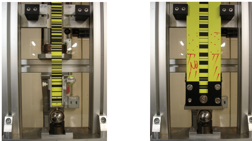
Figure 12: Transfer of offsets from small rods to standard precision rods.
