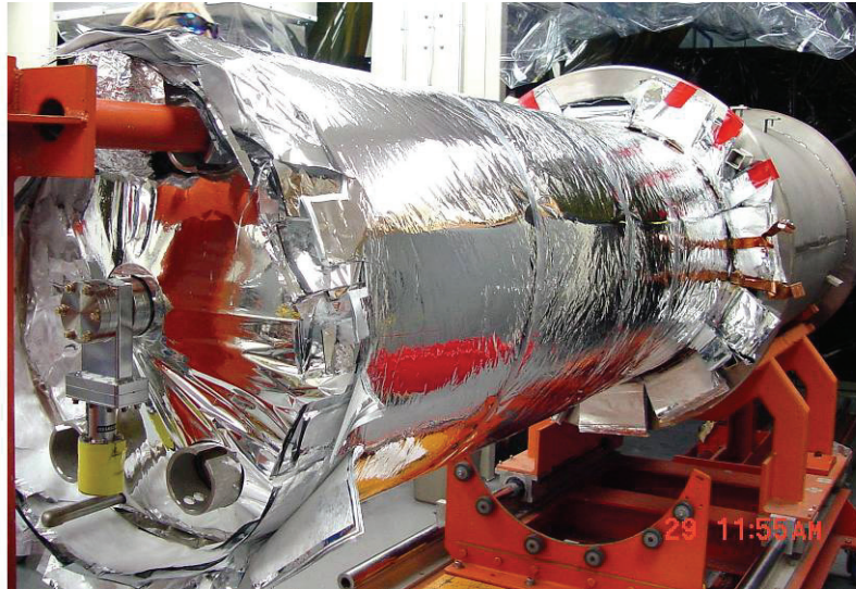
Fig. 3. Helium Vessel inserted into Vacuum Vessel
