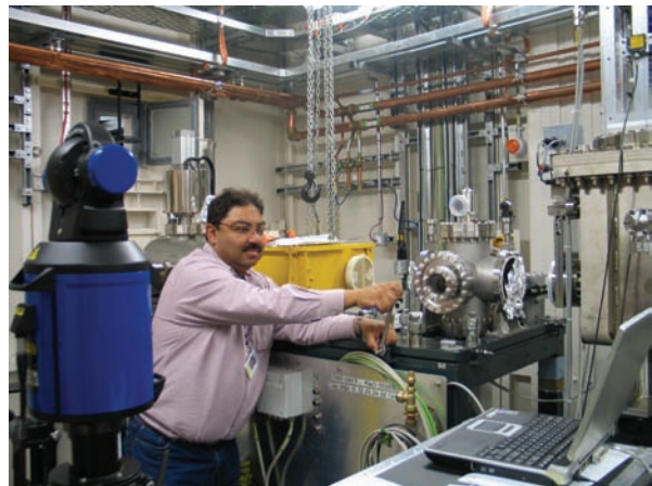
Figure 20: Beamline alignment with laser tracker
