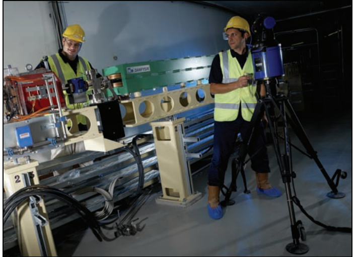
Figure 9: Booster girder alignment
