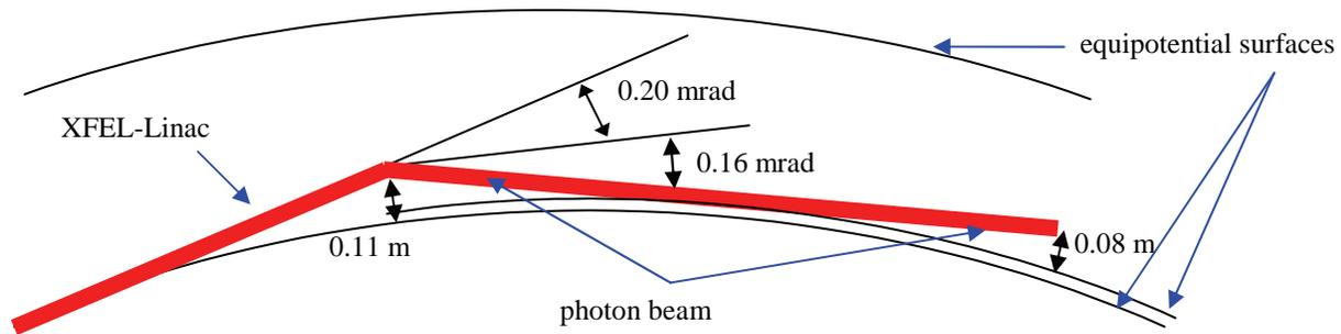
**Figure 8: vertical design of the XFEL tunnel**
