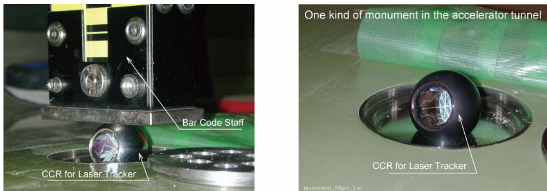
Figure 13 : Floor monuments in accelerator tunnels
