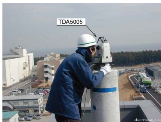
Figure 6 : Surveying for surface network by TS
