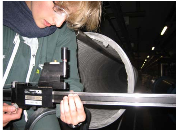
Figure 10 and 11: wire offset measurement system
