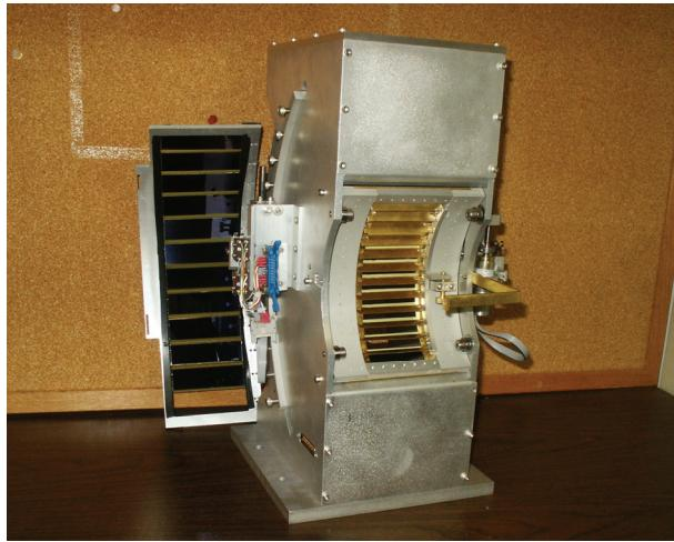
**FIGURE 1.** 12-element multilayer array analyzer detector.
