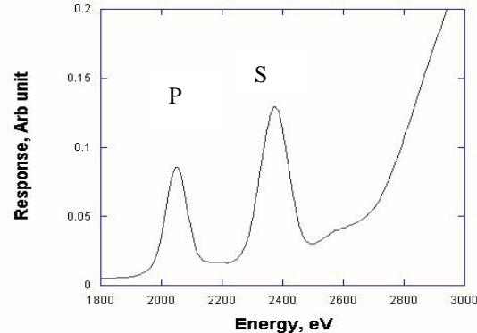
**FIGURE 2.** Fluorescence response on a Bovine liver sample. Note that the multilayer rocking curve has been converted into energy space.
