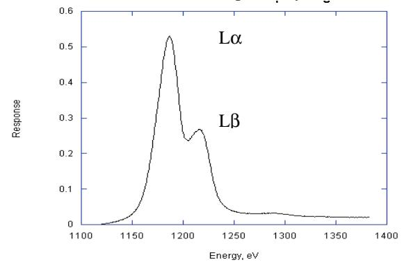
**FIGURE 3.** Detector response at Ge L fluorescence.
