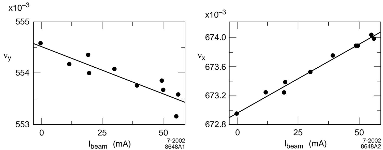
Figure 9: Measured tune variation with current
