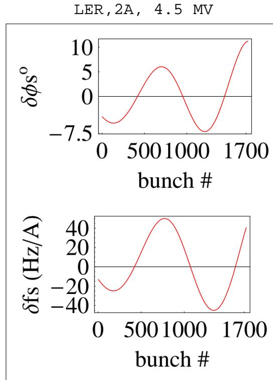
Figure 2: Synchronous phase (top) and synchrotron frequency (bottom) along the train caused by the ion gap.
