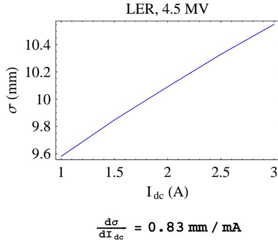
Figure 5: Averaged over the train bunch length vs beam current. Inductance  $L = 80$  nH.
