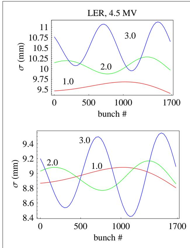
Figure 3: Calculated variation of the bunch length along the train. Bottom plot: results of only gap transients. Upper plot: variation due to the gap transients and the PWD. Beam current is indicated in the figure. LER,  $V = 4.5MV$ . Note increase of the variation with the detuning.
