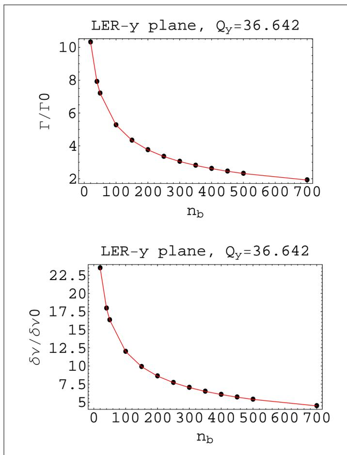
Figure 8: Growth rate and the tune shift as function of the number of bunches for a fixed beam current and bunch spacing.
