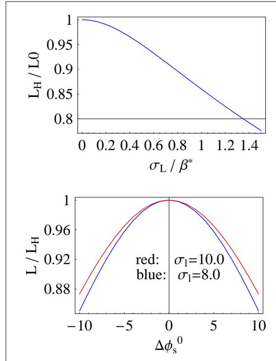
Figure 4: Hour-glass effect (left) and variation of the luminosity with the synchronous phase error (right) normalized to nominal  $L_0$ .  $\beta_y^* = 1.0$  cm. a) hour-glass due to  $\sigma_l$  variation, b) gap transients due to syn. phase variation.
