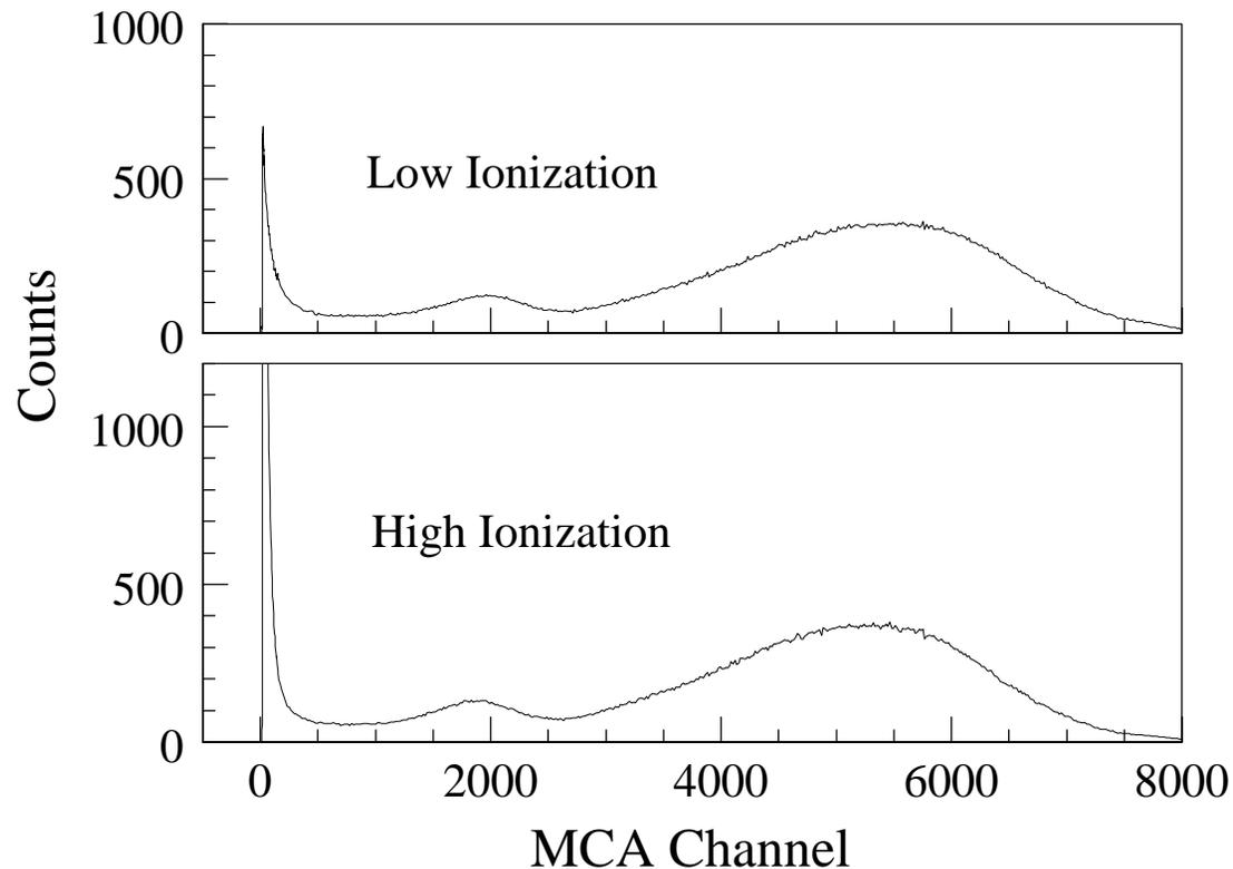
The number of small pulses per  $^{55}\text{Fe}$  conversion is larger at higher ionization levels in an **aged** chamber.
