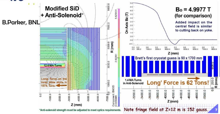
Antisolenoid was recently redesigned, and use of high temperature superconductor was considered. Top ~20-35K would make cooling much easier
