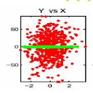
When solenoid overlaps QDO, anomalous coupling increases the IP beam size 30 – 190 times depending on solenoid field shape (green=no solenoid, red=solenoid)
