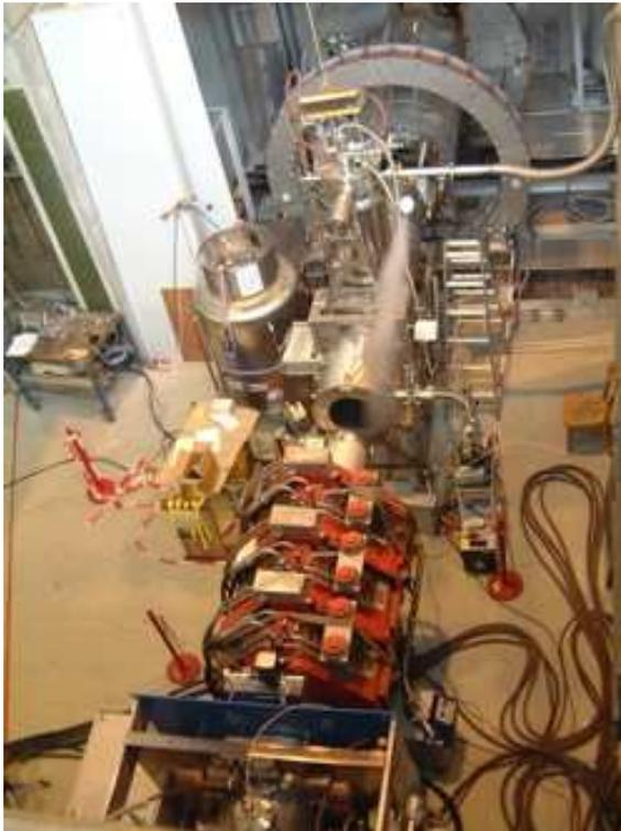
Figure 6: The  $\pi E5$  beam line at PSI. From upstream (bottom) to downstream (top) are the DC separator, the quadrupole magnets (red), the superconducting muon transport magnet, and the COBRA magnet with ring-shaped compensation coils.
