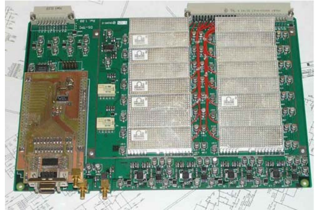
Figure 7: Prototype DAQ board based on the serial converter architecture. Top-right: front-end analogue preamplifiers. Left: digital link. Bottom-right. Delta-sigma converters + gluing logics.
