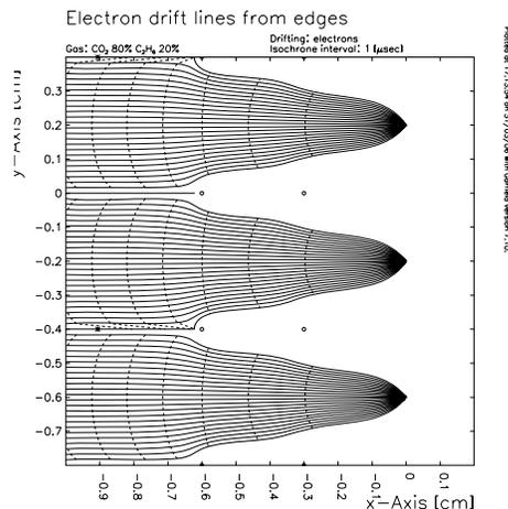
Figure 1: GARFIELD plot of isochronous drift cell, developed from Ref. [22]. The cell consists of three wire planes of equal pitch, two of them for field shaping and the third of anodes. Drift lines and isochrones are shown. The small curvature of the isochrones in the homogeneous field region shows that this arrangement has an extremely linear space-time relation for the  $z$  (drift) coordinate.
