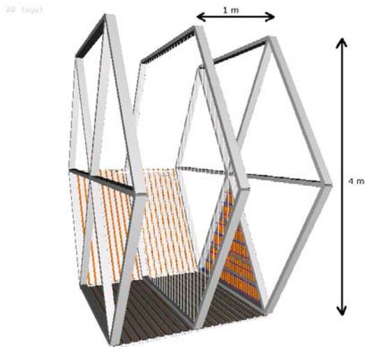
Figure 5: Schematic of 20 m<sup>3</sup> NITPC module discussed in the text.
