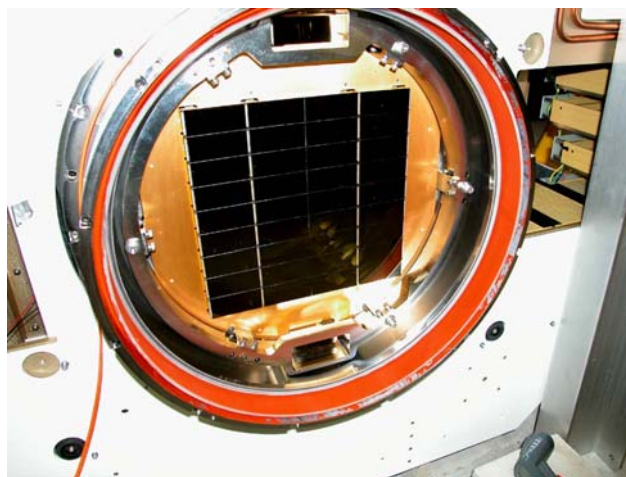
Fig.2. A mosaic with 36 CCDs, 2048x4608 pixels each, in the camera of the SAO Megacam (Courtesy: John Geary).
