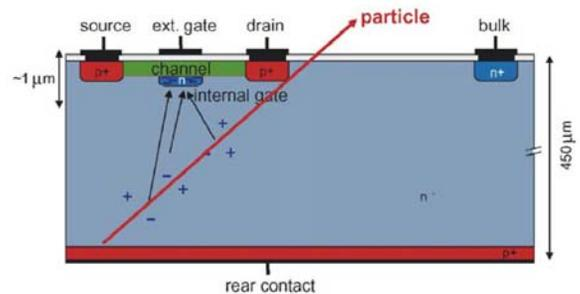
Figure 24. Cross-section of a DEPFET pixel through the transistor channel, illustrating the principle of operation.[40]
