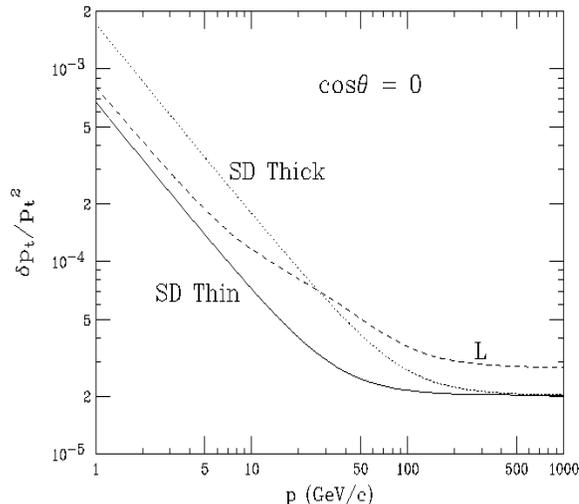
**Figure 25. Momentum resolution of two extremes of a compact silicon tracking system for the ILC, labelled SD Thick and SD Thin in reference to the amount of material in the tracker. For comparison, the resolution of a larger gaseous tracker (L) is shown.[44]**
