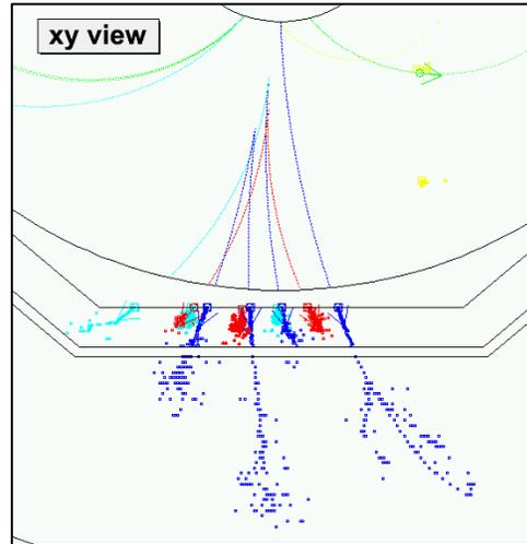
Figure 18. Simulation of jet interaction with calorimeter.[32]
