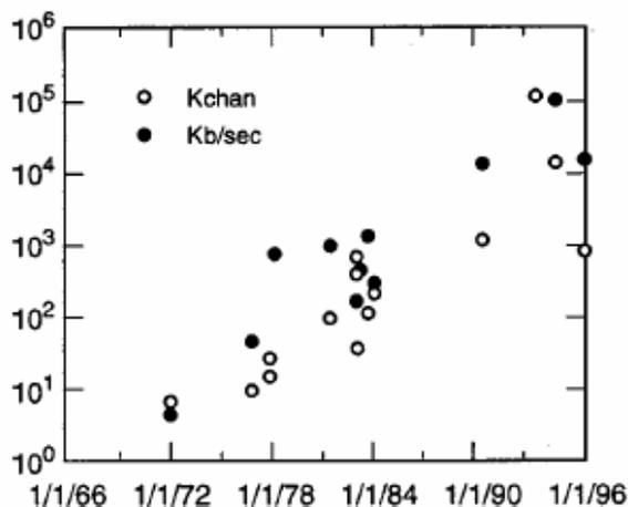
Figure 11. Evolution of the number of detector signal channels with time. Open circles: number of electronic instrumentation channels in thousands; closed circles: design data rate in kilobytes per second to permanent storage. See [19] for details.
