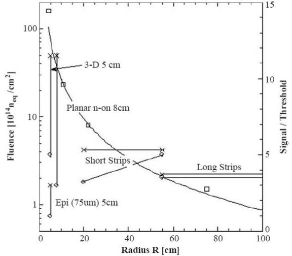
**Figure 21.** The fluence for an integrated luminosity of 2500 fb<sup>-1</sup> as a function of radius R (left scale) is based on the data of open squares, with a fit of the form 1150/R<sup>1.6</sup> superposed. The anticipated signal-to-threshold ratios (right scale) for silicon detectors in the tracker regions with the initial value (x) and that after an integrated luminosity of 2500 fb<sup>-1</sup> (diamond).[22]
