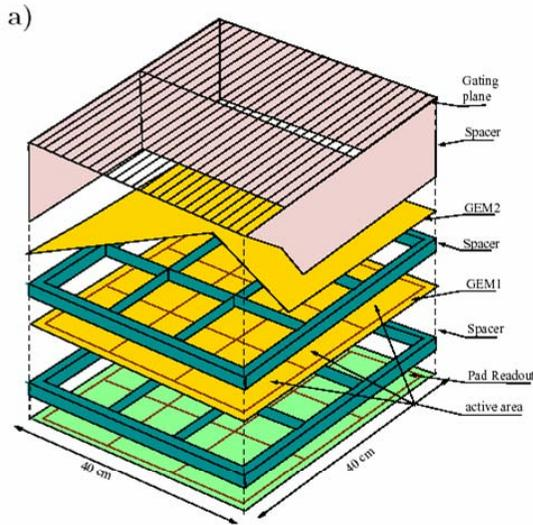
**Figure 27. Schematic of GEM detector.**
