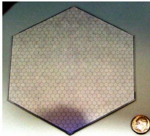
Figure 16. Prototype Si-W EM calorimeter wafer array.[16]
