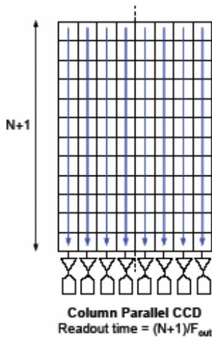
Figure 23. Illustration of a column parallel CCD.[38]
