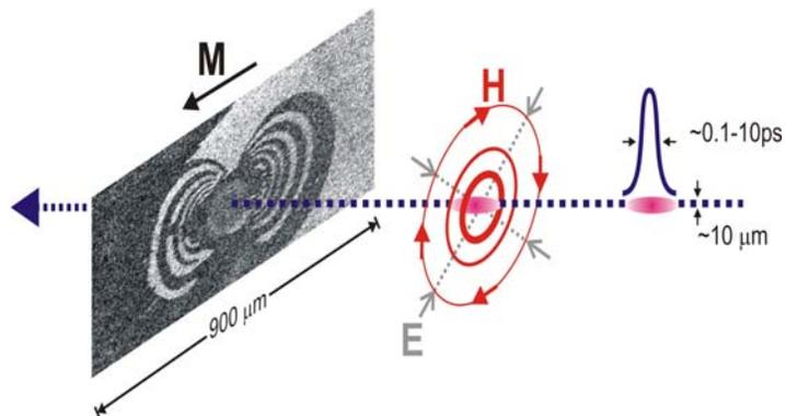
Precession and damping of magnetization in GaAs when exposed to a short pulse electron beam.
