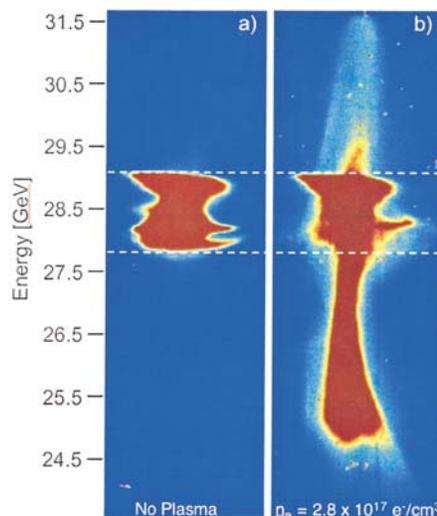
Multi-GeV acceleration of electrons in a plasma wakefield accelerator.
