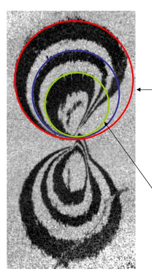
Magnetic pattern of 10 nm Fe film with **167 fs** bunch length Pattern size 470 µm by 980 µm
